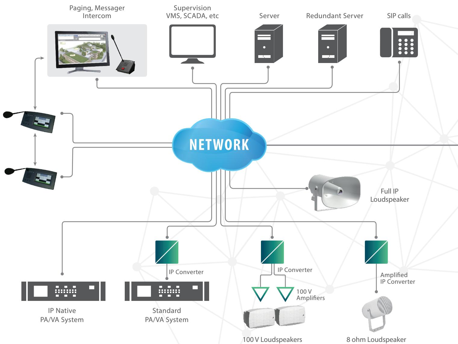
*Vox@net (AMS) manages and controls your audio system over an IP network. No matter the size or location of the sites to be equipped, Vox@net will provide you a full control of your audio system in a simple way.*
