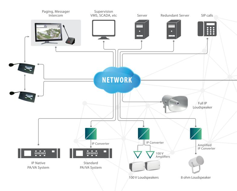
Vox@net (AMS) manages and controls your audio system over an IP network. No matter the size or location of the sites to be equipped, Vox@net will provide you a full control of your audio system in a simple way.
