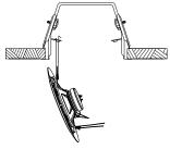
**3) FITTING THE SPEAKER**Compress "V" spring and fit into the retaining ear within the bracket.
