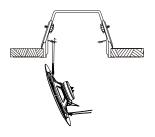
**3) FITTING THE SPEAKER**Compress "V" spring and fit into the retaining ear within the bracket.
