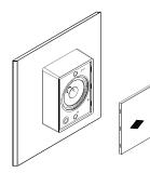
3) Connect the speaker cable into the 3 way terminal block located on the cabinet. Select your required tapping. Fix the speaker cabinet to the wall using suitable fixings (not provided).
