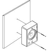
2) Once the grill has been removed place the speaker on a flat surface in your chosen position. Mark the fixing points on the wall. Prepare the wall to take the fixings. If 20mm cable glands are to be used then the speaker cabinet can be drilled using a suitable drill bit. Make sure you place the cable entry in a location that will not prevent the cable from being blocked or restricted by any internal components.
