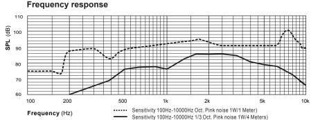
\*Active Equalizer Applied: YES (EQ Setting:+3.5dB@630Hz,+3.5dB@800Hz,-3.5dB@1250Hz,-3.5dB@1600Hz,-2.5dB@4KHz)
